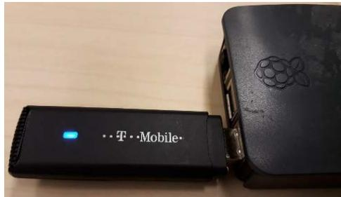
Figure 25. The constant blue light on internet dongle that shows the internet connectivity
