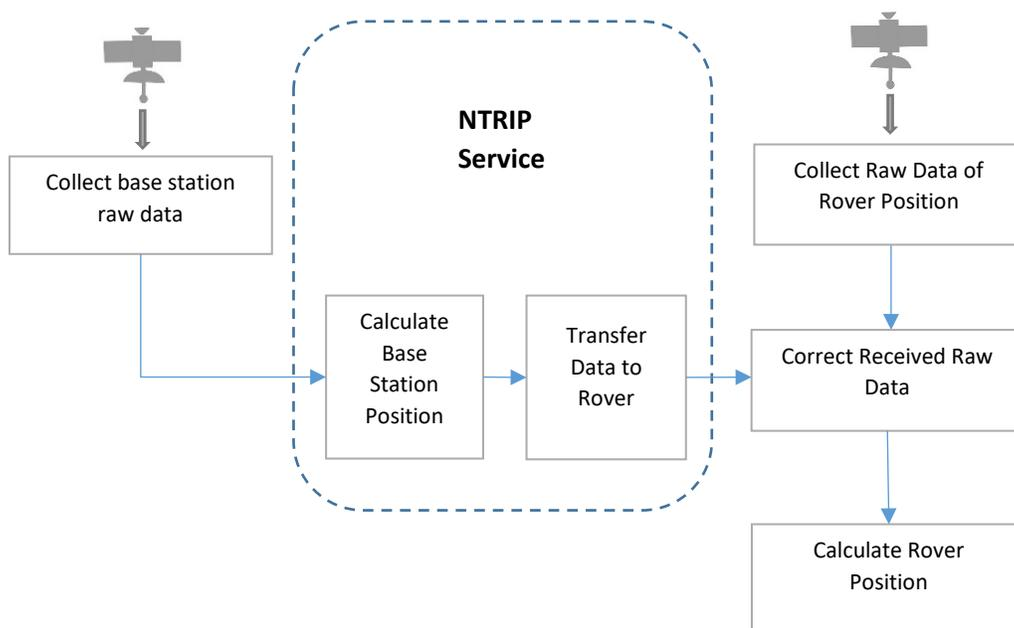
Figure 5. Object positioning based on RTK solution (“Kadaster,” 2018)
