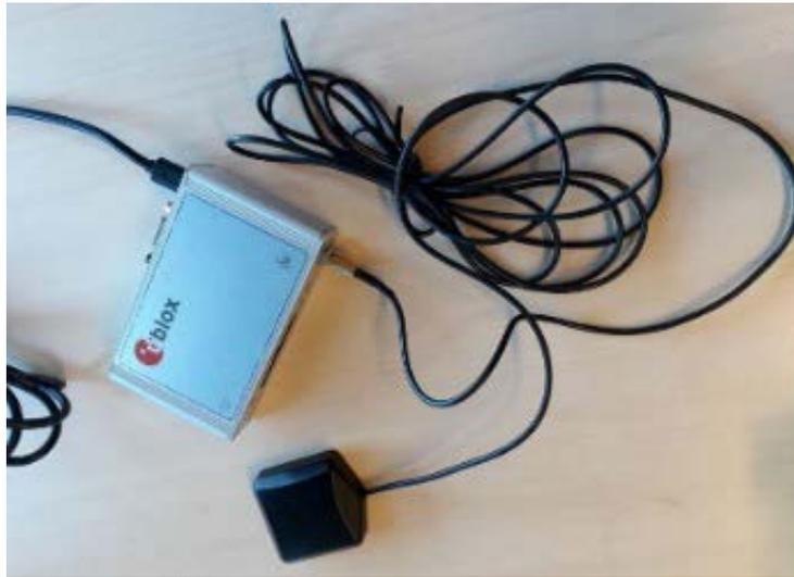
Figure 13. U-blox unit as a component of positioning subsystem
