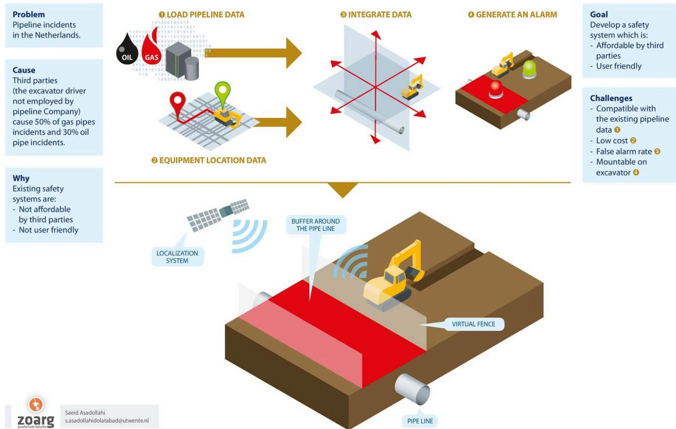
Figure a. The infographic of Geo-fencing based safety system
