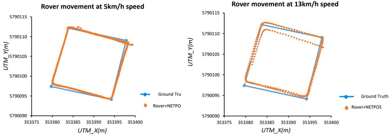
Figure 20. Coordinates distribution compared to the ground truth at 5km/h and 13km/h rover movement speed
