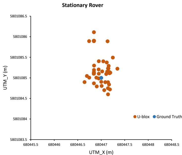
Figure 18. Coordinates distribution compared to the ground truth for a stationary object
