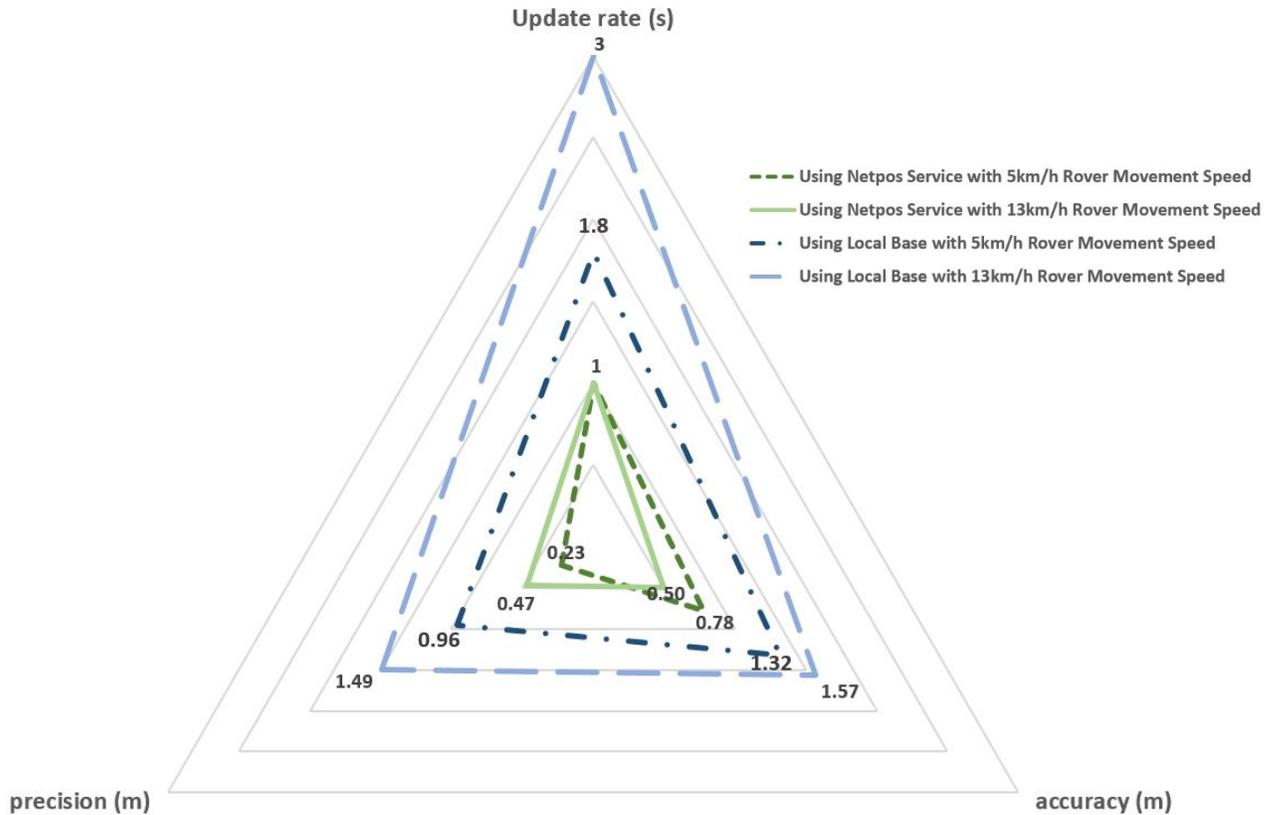
Figure 21. Radar chart of positioning experiment results
