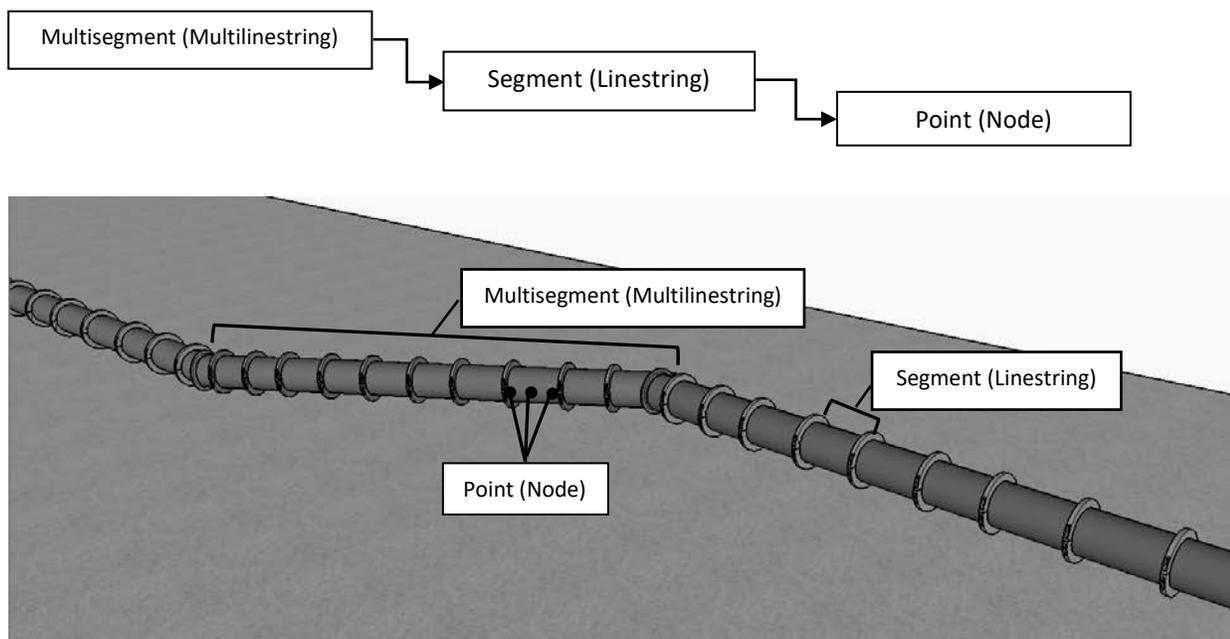
Figure 23. Layers of data in a high-pressure pipelines location file
