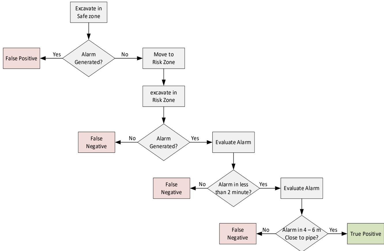
Figure 22. Decision tree to validate generated alarms by the safety system prototype
