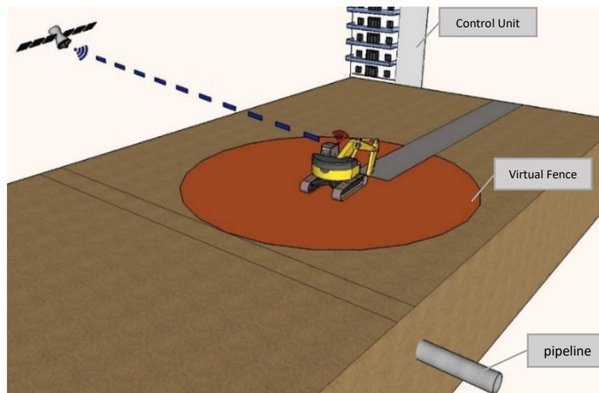
Figure 10. Schematic explanation of a geo-fencing based safety system
