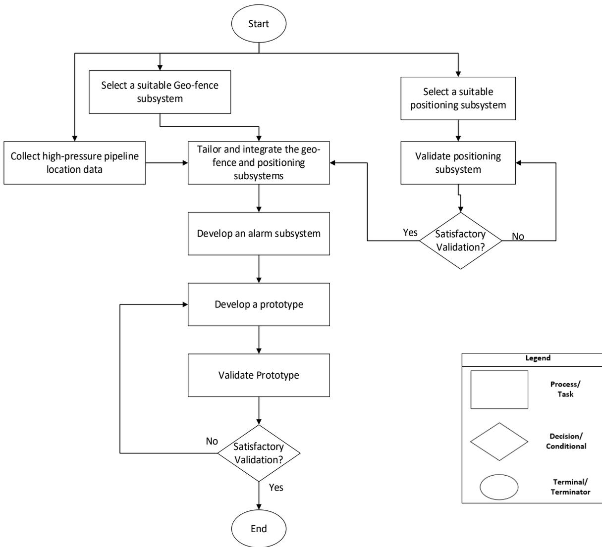
Figure 17. Flowchart of the design procedure
