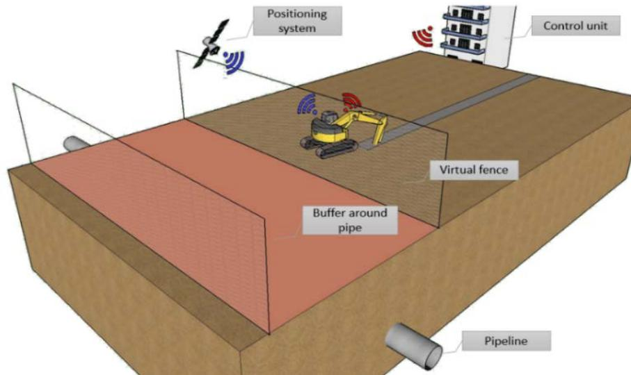
Figure 9. Schematic explanation of initial design of geo-fencing based safety system
