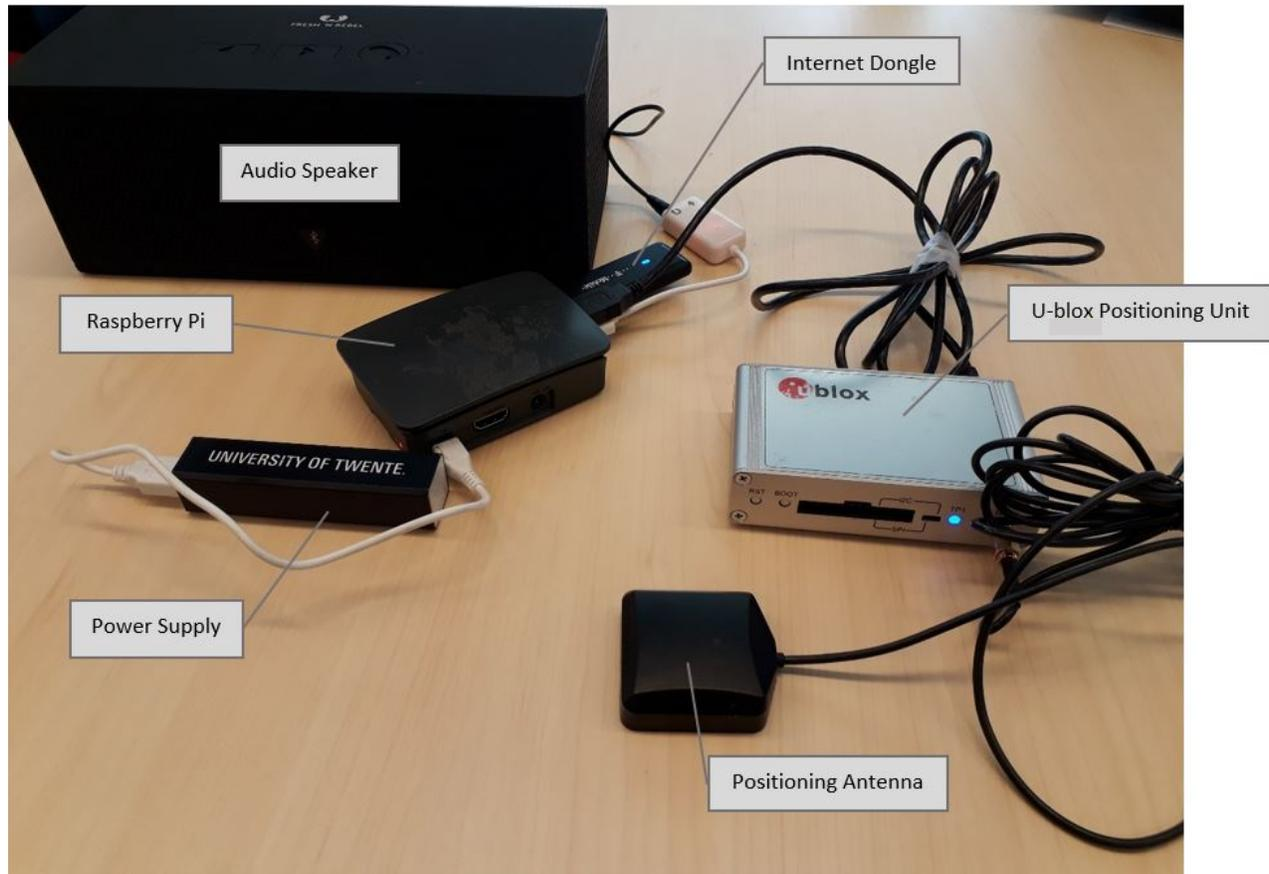
Figure 16. Hardware components of geo-fencing based safety system
