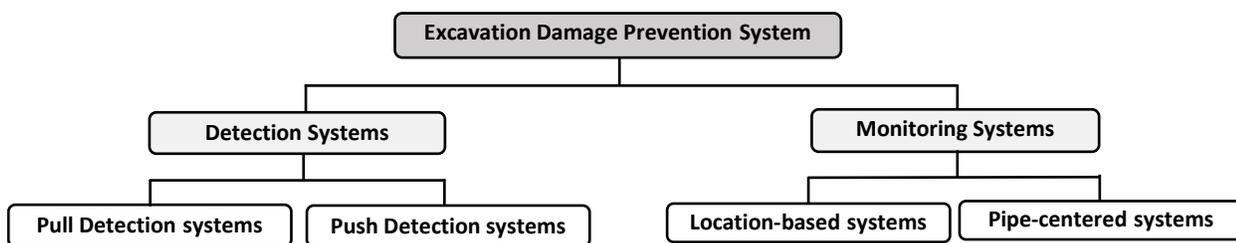
Figure 1. Categorization of the detection and monitoring technologies
