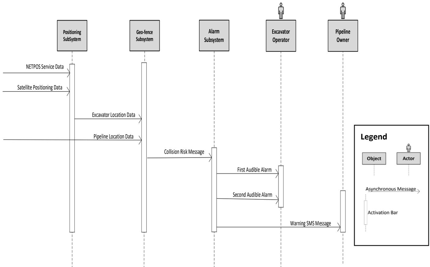
Figure 11. Safety system sequential diagram
